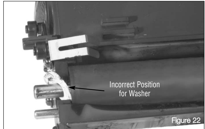
Insert Developer Roller Shaft in to the contact end of the housing.
