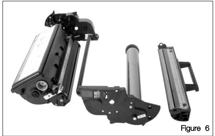
Figure 6 Remove the Drum Idler Gear Axle with needle nose pliers.
